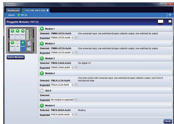
Pluggable modules view simplifies configuration by showing hardware present.
