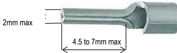
2-17. Lead Terminal for ZEL-C22
