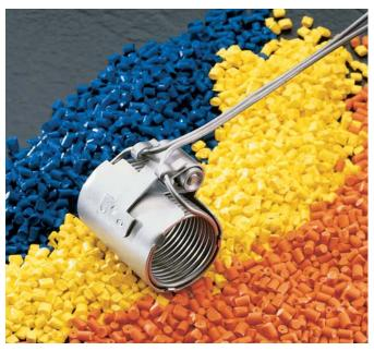
This 0.058-inch diameter heater has been formed into a compact, tightly wound coil to supply 360 degrees of heat. We offer this heater with a 304 stainless steel sheath, the most widely used high temperature sheath material in the industry. It also offers high temperature corrosion and oxidation resistance.
