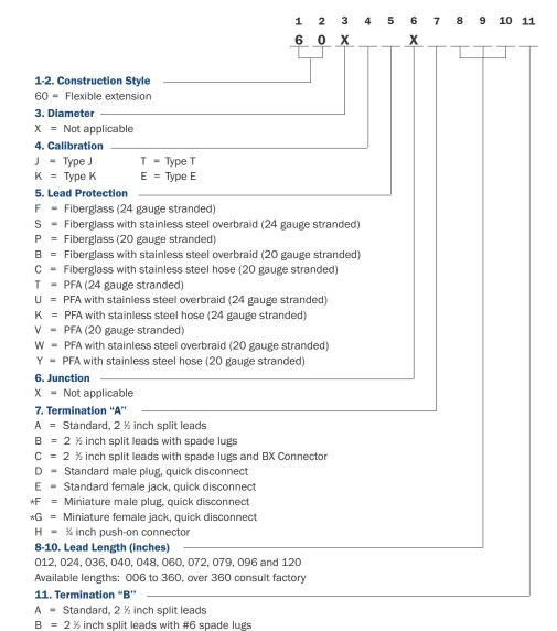
D = Standard male plug, quick disconnect = Standard female jack, quick disconnect = Miniature male plug, quick disconnect G = Miniature female jack, quick disconnect
