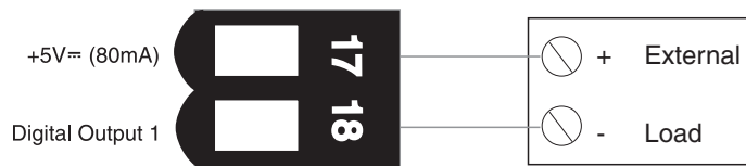
Figure 12.9c — Switched DC Example
