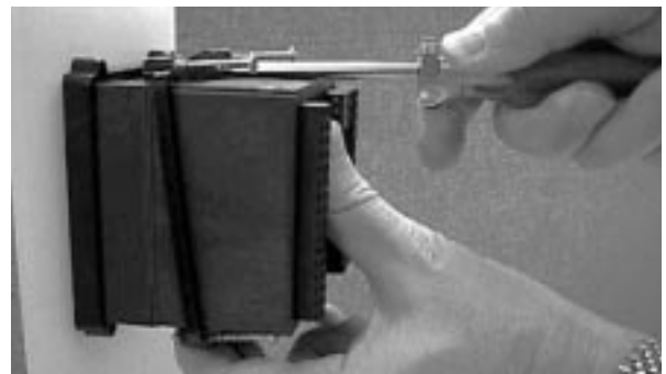
Figure 11.3c — Disengaging the Mounting Bracket.
