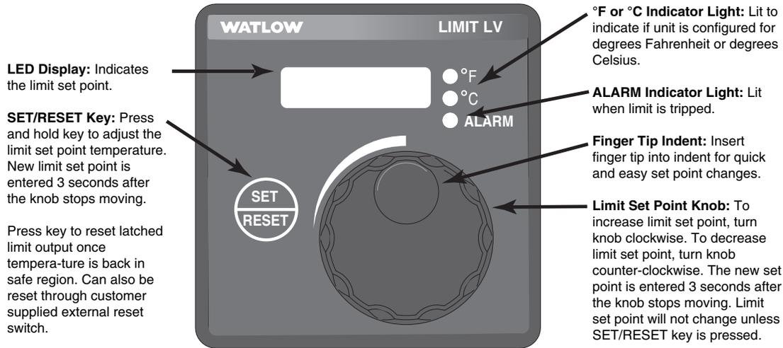
Figure 12 — Variable Limit Set Point, Standard Interface
