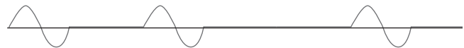
Figure 5.2b — 40% single cycle variable time base 1 cycle on, 1 cycle off, 1 cycle on, 2 cycles off.
