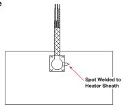
ASTM Type J or K thermocouples are available on lead Type B with loose braid and fiberglass sleeving. They are also available on E, F and H leads. The thermocouple junction, spot-welded to the heater sheath provides a signal for measuring relative heater temperature. A separate thermocouple is available.
