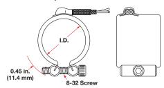
Low-profile clamp bars are available on both 1 in. (25 mm) and 1½-in. (38 mm) wide heaters. For wider widths, contact your Watlow representative. Low-profile clamping on diameters and widths greater than 3 in. (76 mm) is not recommended. The bars are ¼ in. (6 mm) diameter with an 8-32 screw. To order, specify **low-profile clamp bars.**
