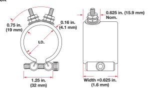
Post terminals provide optimum connections. Screw thread is 10-24. To order, specify **post terminals** (metric threads are available).
