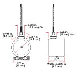
Type K: Flexible lead wires exit vertically from the heater and can be bent adjacent to the heater for a quick, easy connection. To order, specify **Type K** and **length**.
