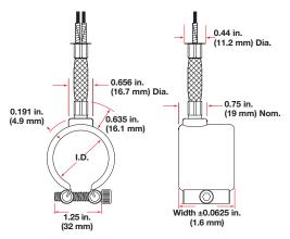
Type E: A loose metal braid encloses two fiberglass leads providing good abrasion protection, lead flexibility and wiring convenience. Leads are 2 in. (51 mm) longer than the braid and are shipped with 12 in. (305 mm) leads, unless a longer length is specified. To order, specify **Type E** and **length.**
